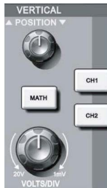
Figure 1-6 Vertical Control Area on the Panel
