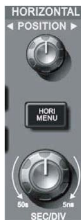
Figure 1-7 Horizontal Control Area on the Panel
